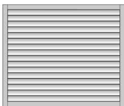
HORIZONTAL LOUVRE INFILL 58MM, 80MM OR 120MM
