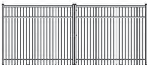
SLIDING GATE 1800MM HEIGHT CONFIGURATION
